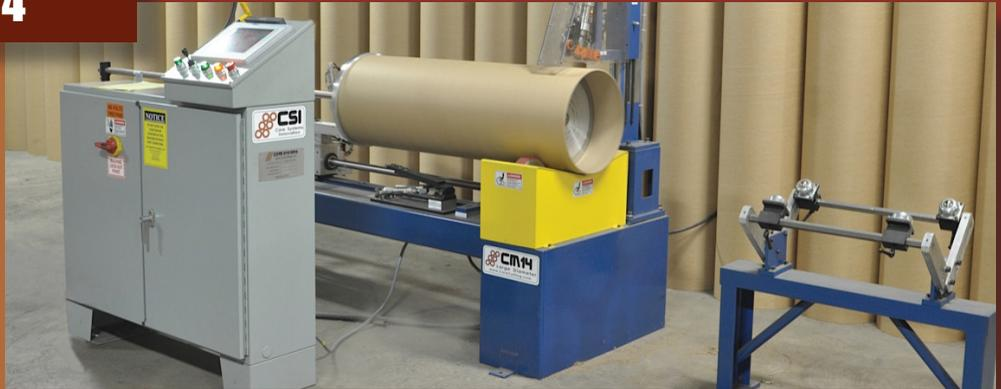
*Western Container, from Beloit, Wisconsin, has launched a new addition to their production capabilities. The CM-14 has recently been added to the manufacturing line to meet the needs of large precision re-cutting. The CM-14 is a heavy-duty automatic core cutter designed to cut cores with large internal diameters with ease and speed.*
